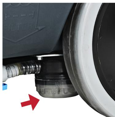
3 Check if the solution filter is cleaned.
