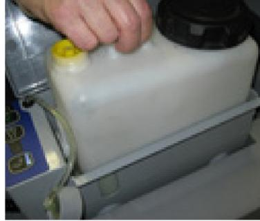
3. Install the detergent bottle suitable for the work to be performed
