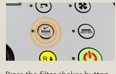
Press the filter shaker button to clean the filter. Hold the button until the light blinks to enable automatic shaking every 10 minutes.
