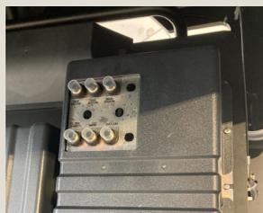
5. Check the vacuum and filter shaker circuit breakers.
