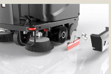
Remove, clean and inspect the main broom and check the side brooms. Clean the machine with a wet cloth.
