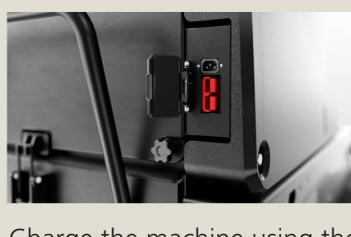
Charge the machine using the rear charging connection. It has two connections, one for external charger and one if on-board charger is installed.
