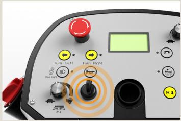
Insert the operator key, and turn to start the sweeper.
