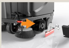
1. Inspect the main broom, make sure it's turning and is not worn out. Adjust broom pressure if needed.
