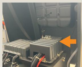
3. Open the machine cover and check the broom circuit breakers.
