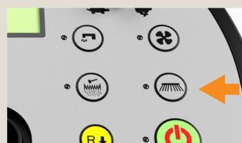
Press the side broom button to lift the side brooms and use the machine with only main broom.
