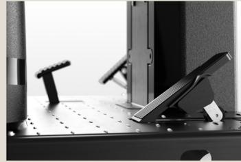
The brushes and vacuum will start when the drive pedal is pressed, start sweeping.
