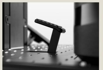
Press the front flap pedal to open the front flap for sweeping larger debris.
