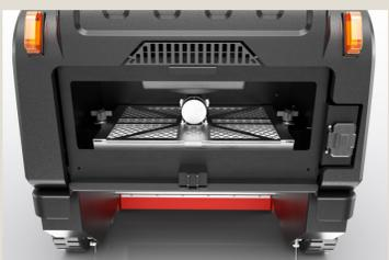
Remove the rear filter panel to check the filter, reinstall panel and hopper.
