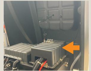
5. Open machine cover and check so no fuses have tripped.
