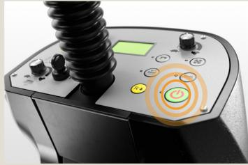
Press the OneTouch™ button to enable all sweeping functions, the brooms will lower automatically.
