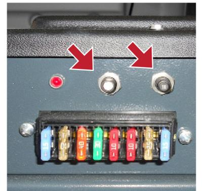
4. Check if the main broom circuit breaker (FA) or the side brooms circuit breaker (FB) is not open.
