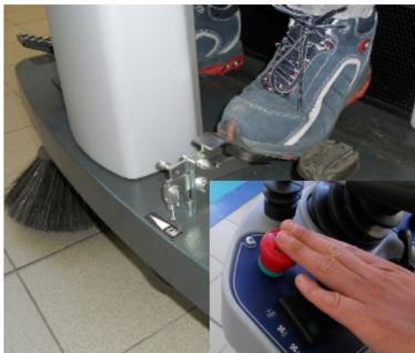
12. Stop the machine by press the service brake pedal. Press the emergency push-button in case of emergency and to immediately stop the machine functions.
