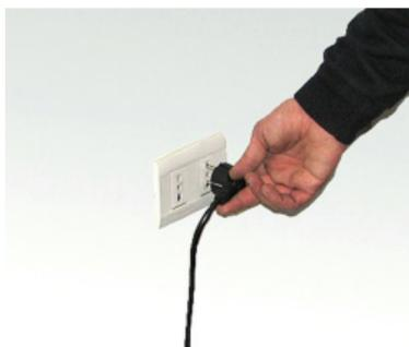
18. (If machine equipped with OBC) Connect the charger cable to the electrical main.
