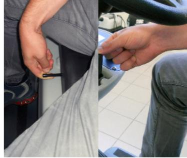
4. Adjust the seat by using the lever. Use the lever to tilt the steering column to a comfortable position.
