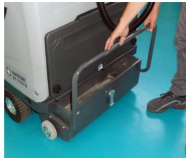
14. Remove the hopper by using the handle and by disengaging it from the inner guides. Discharge all the debris into special containers.
