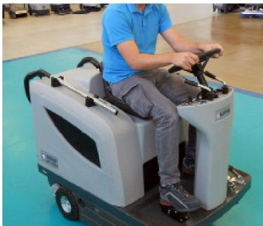
7. Drive the machine by keeping the hands on the steering wheel and pressing the pedal on the front side to move forward and on the rear side to move backward.
