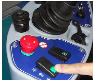
9. Turn on the vacuum system by pushing the switch backward.
