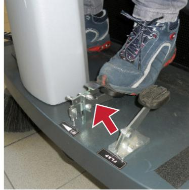
3. Check if the parking brake pedal is disengaged.
