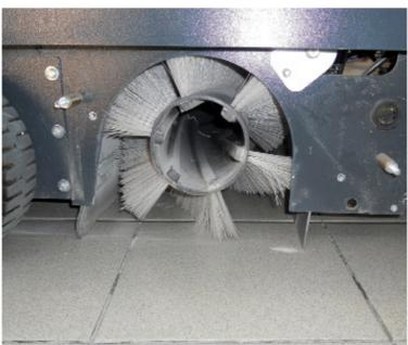
16. WEEKLY: Check the main and side brooms and remove any debris like straps, rope etc.
