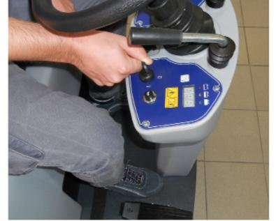
5. Turn the ignition key to "I" and do not press the pedal.
