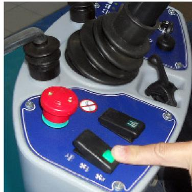
2. Check if the vacuum system switch is on.
