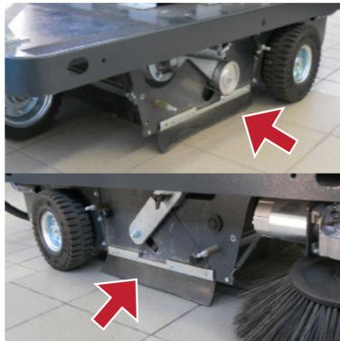
1. Check if all flaps is correctly adjusted and not worn out.
