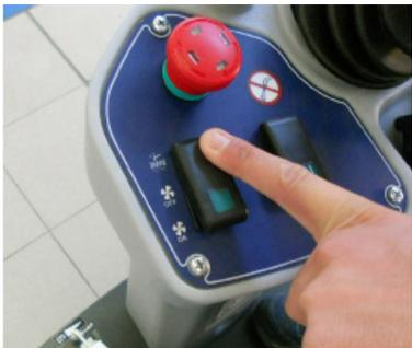
11. To clean the filter, turn on the filter shaker by pressing the switch forward for a few seconds.
