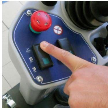
3. Clean the panel filter by pressing the filter shaker switch.
